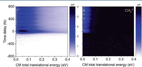
Time-dependant low KER oscillatory structure at positive pump-probe delays.  $\text{CH}_3^+$  yield decreases while  $\text{I}^+$  yield increases with pump-probe delay.
