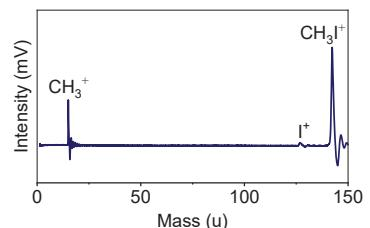
Increased  $\text{CH}_3^+$  signal. The  $\tilde{\Lambda}^2A_1$  state dissociates via internal conversion to the hot vibrational bands of the ground state leading to  $\text{I}^+ + \text{CH}_3^+$ .
