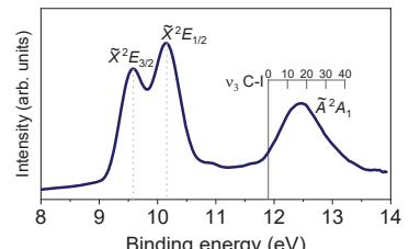
The cation is prepared in the  $\tilde{\chi}^2E_{3/2, 1/2}$  states and in the  $\tilde{\Lambda}^2A_1$  state with high vibrational content ( $v=15$ ).
