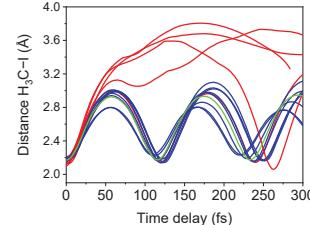
Trajectories show that the wave packet mainly remains in the  $\tilde{\Lambda}^2A_1$  state oscillating (blue lines), while a minor fraction has enough energy to dissociate into  $\text{CH}_3 + \text{I}^+$  (red lines).
